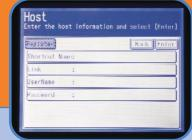
scan to FTP. Files that are too large to be sent via a traditional e-mail server can be scanned to a password protected FTP site for either storage or sharing. Up to 20 FTP shortcut keys can be created for seamless one-touch scan initiation.
